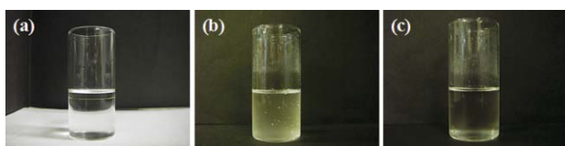
Fig. 4 Photographic observations of emulsification and de-emulsification of allyltrimethylsilane in EMIM BF 4 . (a) Before acoustic emulsification, (b) right after acoustic emulsification, and (c) after 60 min.
